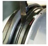
Recheck air gap next to each mounting screw to ensure even adjustment. Repeat as necessary to obtain proper air gap.
