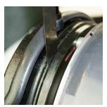
Check the air gap using a 0.8mm feeler gauge referring to the picture below and brake part diagram. The acceptable air gap range is from 0.9mm to 0.8mm. If the air gap is outside the acceptable range continue to step 3 below to perform adjustment.
