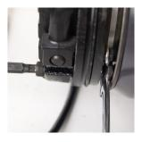
Adjust the brake mounting hollow screws to obtain proper air gap. Only small adjustments should be required.
