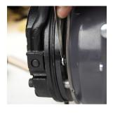
Check release handle air gap at position "S".
