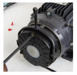
Loosen the brake mounting screws.
