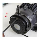
Tighten brake mounting screws.
