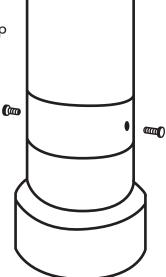
To remove lift piece, remove the two side screws holding it in place.
