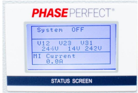
Figure 24 – “System Off” Status Screen
