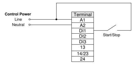
Figure 3 - Control via 2-Wire Start/Stop
