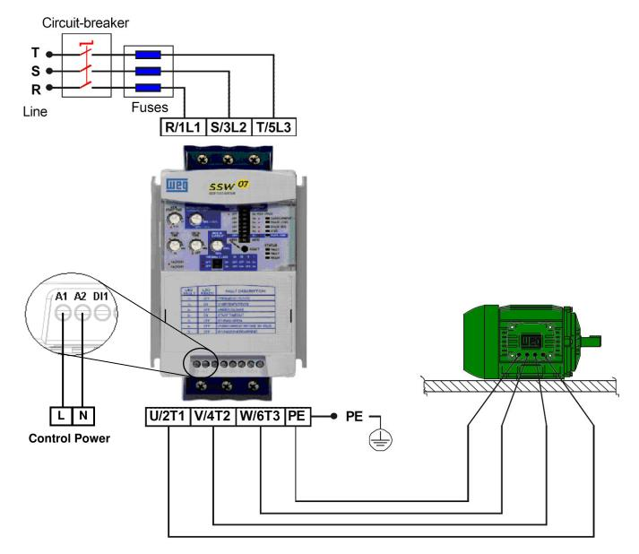
Figure 1 - Power and Grounding Connections
