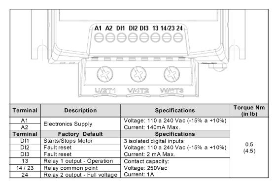
Figure 2 – Control and Signal Connections
