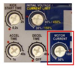
Figure 6 – Motor Current Trim-Pot Location
