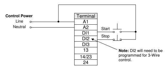
Figure 4 - Control via 3-Wire Start/Stop
