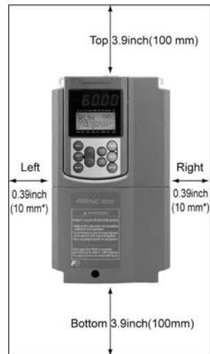
Figure 2.1 Mounting Direction and Required Clearances
