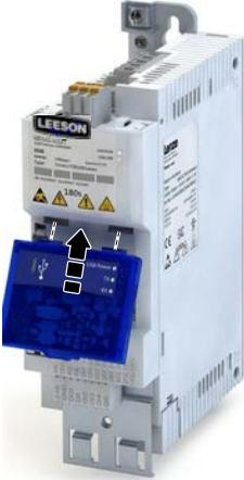
2. Turn it downwards until it engages into the lower mounting slot.
