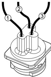
**For grounded tools with 3 wire Quik-Lok cords:** Orient the pin housing assembly as shown and place white wire #2 first into bottom of handle portion of motor housing.
