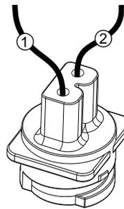
**For double insulated tools with 2 wire Quik-Lok cords:** Orient the blade housing assembly as shown and place white wire #2 first into the bottom of handle portion of motor housing.
