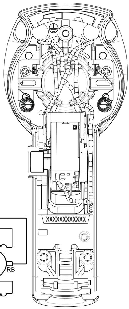
**AS AN AID TO REASSEMBLY, TAKE NOTICE OF WIRE ROUTING AND POSITION IN WIRE GUIDES AND TRAPS WHILE DISMANTLING TOOL.**
