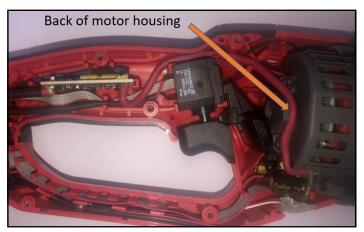
Route the two thin black wires through trap at the back of the motor cage. Place the large red wire over the thin wires in that trap. Continue routing large red wire as shown.
