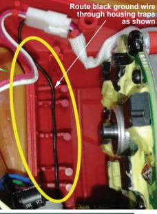
As an aid to reassembly, take notice of wire routings and position in wire guides and traps while dismantling tool.
