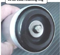
add new 44-86-1400 self-locking retaining ring over existing 44-86-1380 retaining ring with its concave side facing the -1380 retaining ring
